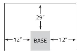
Using a 3/8" Masonry Bit, drill through the four holes in the stand base into the cement floor to mark hole locations. Remove the stand and complete drilling the four holes to a depth of 4". Use a vacuum cleaner to remove cement dust from holes.
