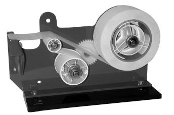
The Double Sided Grip Tape Dispenser accepts tape up to 2" in width. It makes handling grip tape simple and hassle free by removing the paper liner and winding it onto a spool as you use the tape.
