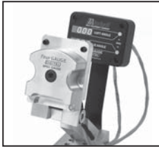
Putter Loft/Lie Angle Gauge Assembly (#1)
